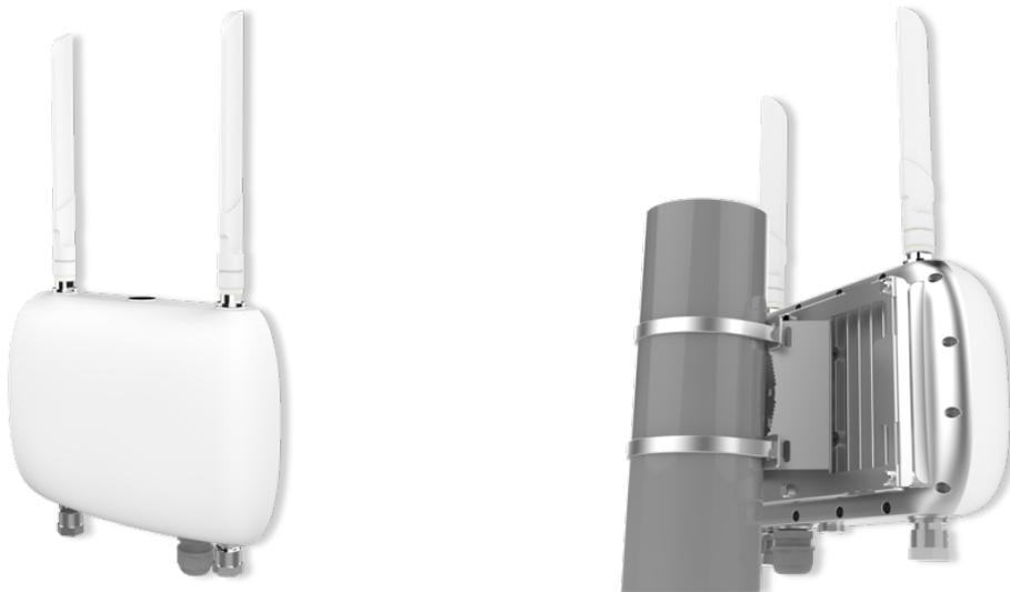
This outdoor gateway uses LoRaWAN technology from Semtech and is complied with specification defined by LoRa Alliance. This gateway has two LoRa, one GPS & one LTE antenna ports and is powered through 48 VDC PoE. Its LoRa interface operates in 863-870 MHz band and supports end-devices with class A & C, Listen Before Talk, Spreading Factor, Adaptive Data Rate (ADR), GPS Timing and Geo-Localization Service.
